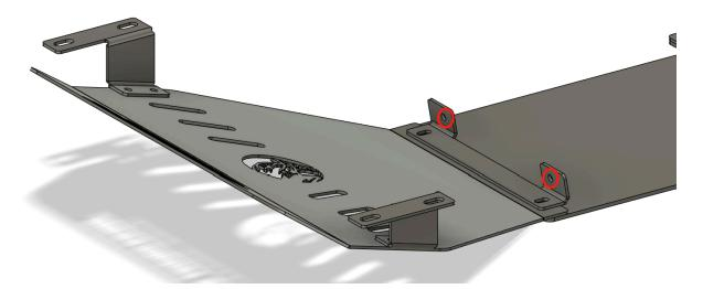
4. Next install the provided % clip nut on the passenger side of the crossmember in the location shown below. The clip nut can be installed from the outside of the crossmember and slid until the threads align with the pre-existing hole in the crossmember.
