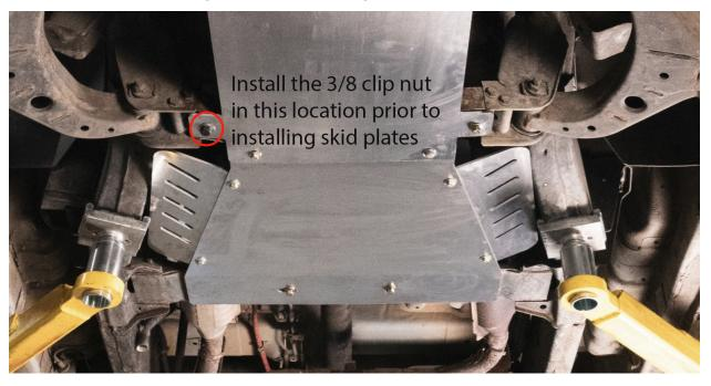
5. With the brackets and clip nut installed you can now mount the front and middle skid plates. Use the provided % grade bolts, washer and nylock nuts to install the skid plates in the locations shown below.
