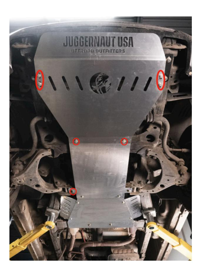
6. Next use the provided M12-1.75x80mm flange bolt and nut to secure the drivers side of the skid plate through the existing hole in the crossmember in the location shown below.
