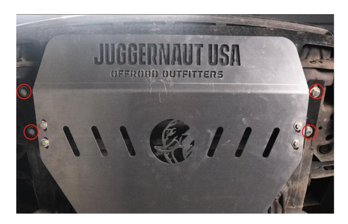
3. The next step is to attach the rear bracket for the front skid plate. Using the provided (2) M8-1.25x25mm bolts and washers attach the bracket to the subframe crossmember in the locations shown below. There will be threaded holes in the subframe that will line up with the bracket.
